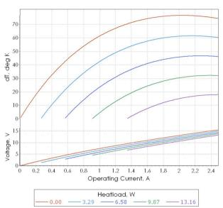
**Note**: Performance data is specified for optimal optimal conditions (TEC hot side is stabilized at ambient temperature). Heatsink thermal resistance is not included into estimations. Use TECCad Software for estimations under different conditions.
